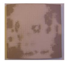
Fig 26 Substrate (layer 2-without carbon) produced using compression pressure of :150Bar, Sintered at 1400C for 6h
