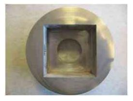
Fig 39 One of the previous dies (female part) manufactured for substrate fabrication
