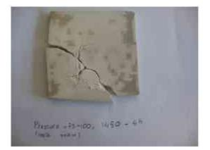
Fig 23 Substrate (layer2) produced using compression pressure of  $\approx$  90Bar, Sintered at 1400C for 4h
