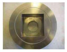
Fig 40 Last die (female part) for substrate fabrication
