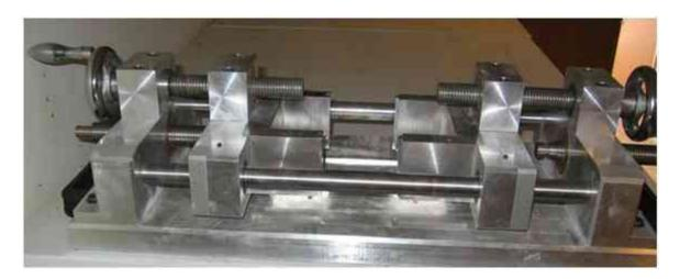
Fig 43 A different version of the die which can be adjusted according to desired substrate size
