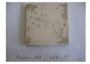
Fig 18 Substrate (layer 2) produced using compression pressure of :150Bar, Sintered at 1450C for 6h
