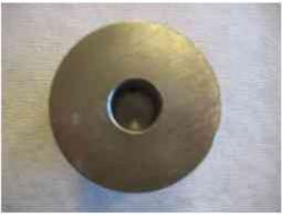
Fig 41 One of the previous dies manufactured for pellet fabrication
