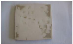
Fig 16 Substrate (layer 2) after sintering
