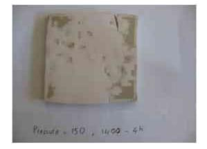
Fig 19 Substrate (layer 2) produced using compression pressure of :150Bar, Sintered at 1450C for 4h
