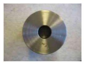
Fig 42 Last die used for pellet fabrication
