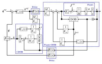
Fig. 5. A block diagram of a proposed position/force hybrid control system
