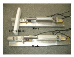
Fig. 11. The bilateral master/slave robots
