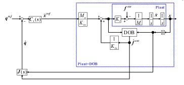
Fig. 2. A block diagram of a position/force hybrid control system
