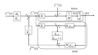
Fig. 1. A robust acceleration control using DOB
