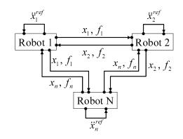
Fig. 3. The conventional structure for a hybrid control system with multiple plants
