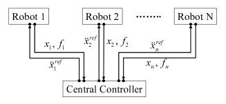
Fig. 4. The proposed structure for a hybrid control system with multiple plants
