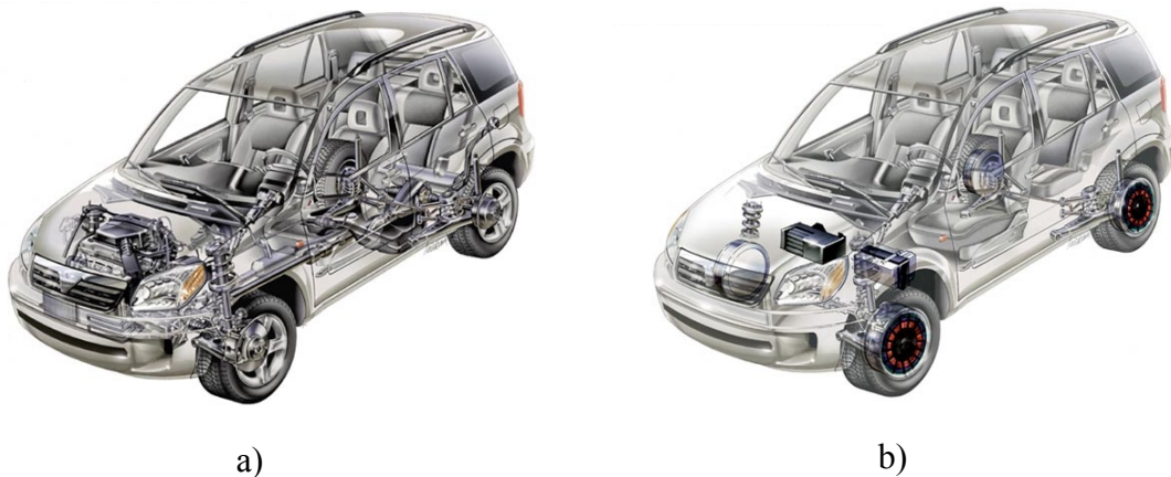
Figure 1.2 : An Example of how In-wheel Motor concept can revolutionize the vehicle design concept; a) Conventional 4 Wheel Drive Vehicle, b) New configuration using Wavecrest Adaptive In-wheel motors
