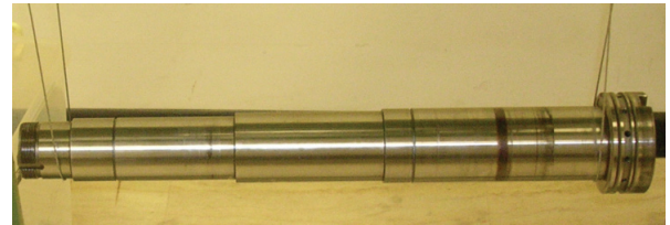
Figure 4: Spindle suspended for free-free measurements.
