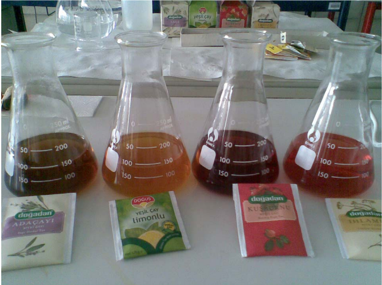
Picture 9 (above): The colours of the tea solutions after they are being titrated. From left to right, you see Sage Tea, Green Tea with Lemon, Rosehip Tea and Linden Tea. After the titration, Sage Tea becomes dark brown, Green Tea becomes reddish-brown, Rosehip Tea becomes nearly black and Linden Tea becomes pink.
