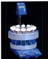
Figure 1.18 Carousel reactor for high-throughput method.
