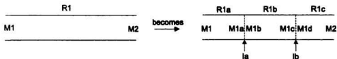
Figure 7.1: A road model to allow three robots to travel within R1 simultaneously.
