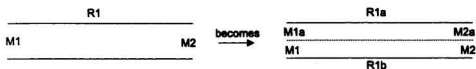
Figure 7.2: A road model that will allow two-way travel in a road segment.
