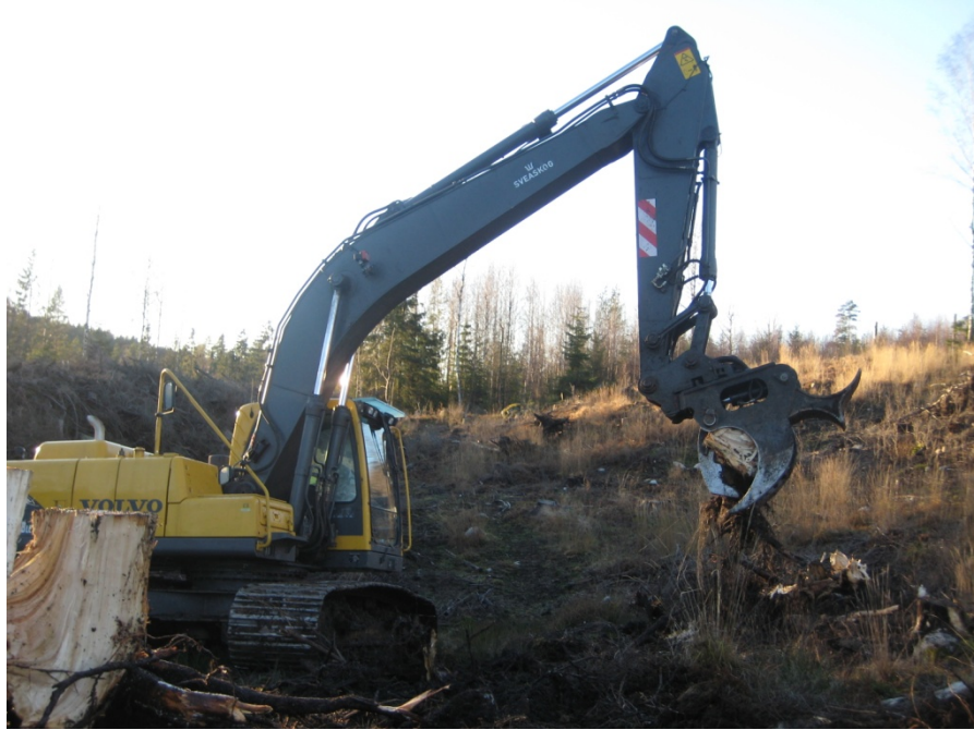
Figure 1. Stump extraction in the stump harvest catchment study (paper II). Photo: Kevin Bishop
