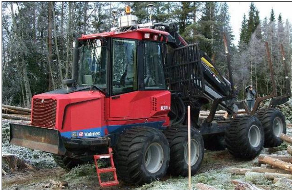
Figure 1. The studied Valmet 830 forwarder equipped with an RTK DGPS for localization and heading measurements and a gyro determining the vehicle's roll and pitch angles. Photo: Ola Ringdahl.
