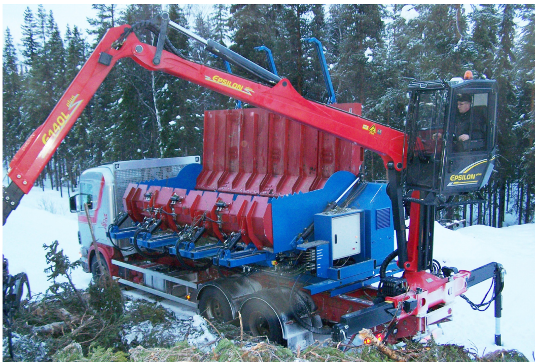
Fig. 1. The studied prototype machine (Rogbico GTK 4800). Note that the loading chamber is not pivoted towards the windrow in the picture.
