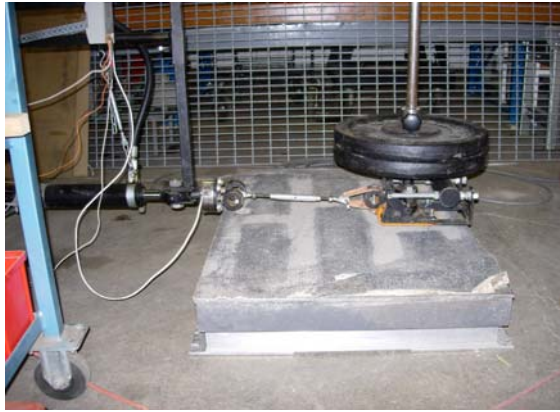
Figure 11. The PSM friction measurement device (at FP calibration set-up).
