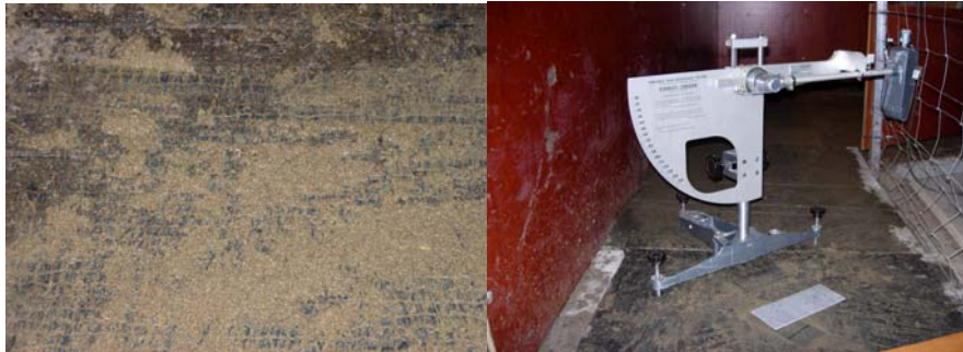
Figure 9. Fouled rubber floor mat KEN ® (left) and SRT friction measurement device on FP flooring (right).
