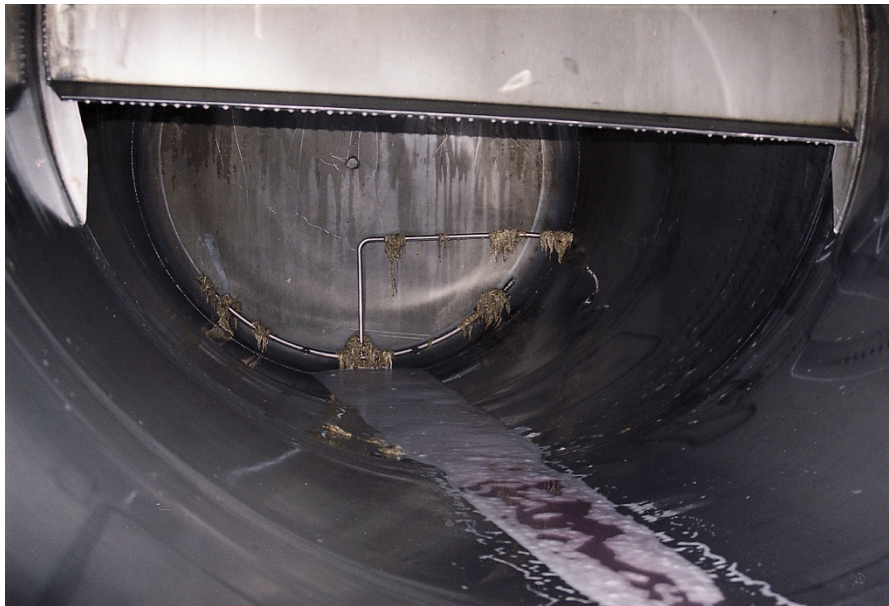
Figure 12. Inside of a tank after cleansing and disinfection. Manure can be seen in the tank. (Photo: Nils-Gunnar Ericsson, November 2004)
