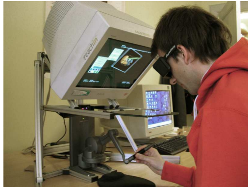
Figure 5.2: A workstation for interactive segmentation of volume images, featuring a 3D input device with haptic feedback and a stereoscopic display.
