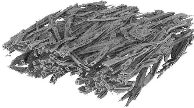
Figure 5.1: A surface rendering of fibres in a pulp-fibre composite material, captured with \mu CT. The polymer matrix surrounding the fibres is not shown.
