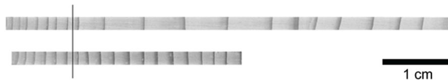
Fig. 2. Two fibre property samples from Flakaliden; IL, upper and C, lower, view from above. Vertical line marks the annual ring formed in 1987, the first year of treatment.
