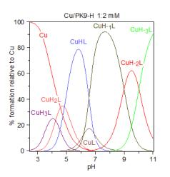
Fig. 1 Exemplificative distribution diagram for the system Cu(II)/peptide 1
