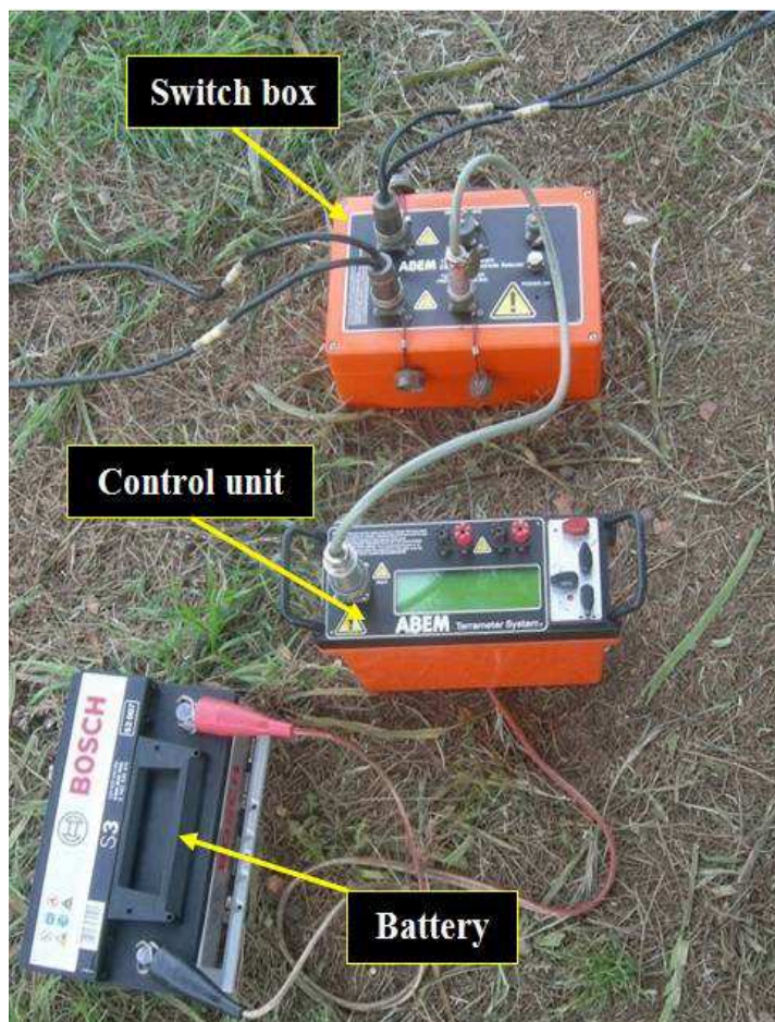
Fig. 1.9 - Arrangement for data acquisition with Abem Terrameter SAS1000 and Lund 2D multi - electrode resistivity survey.
