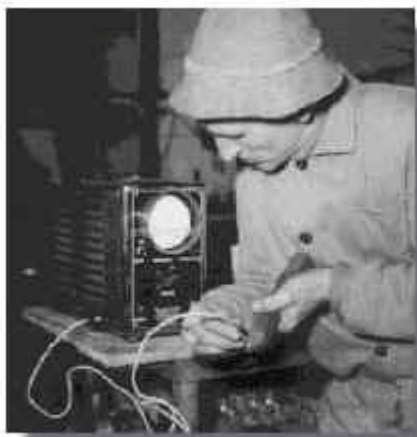
The ultrasonic Reflectoscope in use** ( Courtesy of KretzTechnik, Austria )
