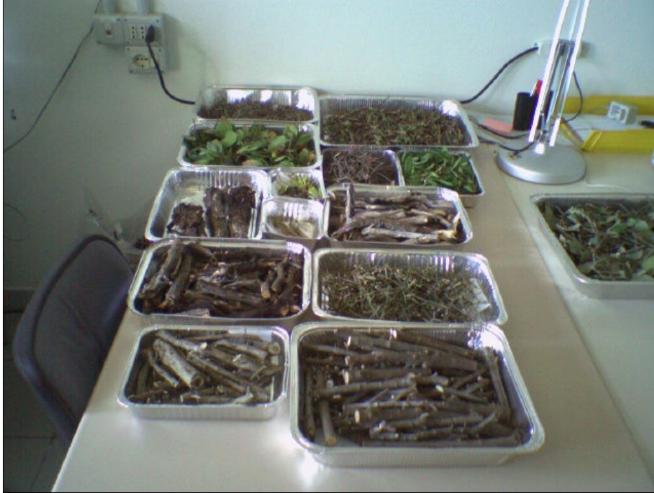
Figure 51. Samples of live and dead fuel, divided in timelag size classes, before the oven dry at 102 °C
