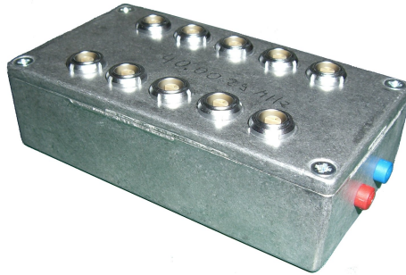
Figure B.42: Picture of the 40 MHz clock. The device needs +5 V. The clock can be distributed to up to 10 TacQuilas.
