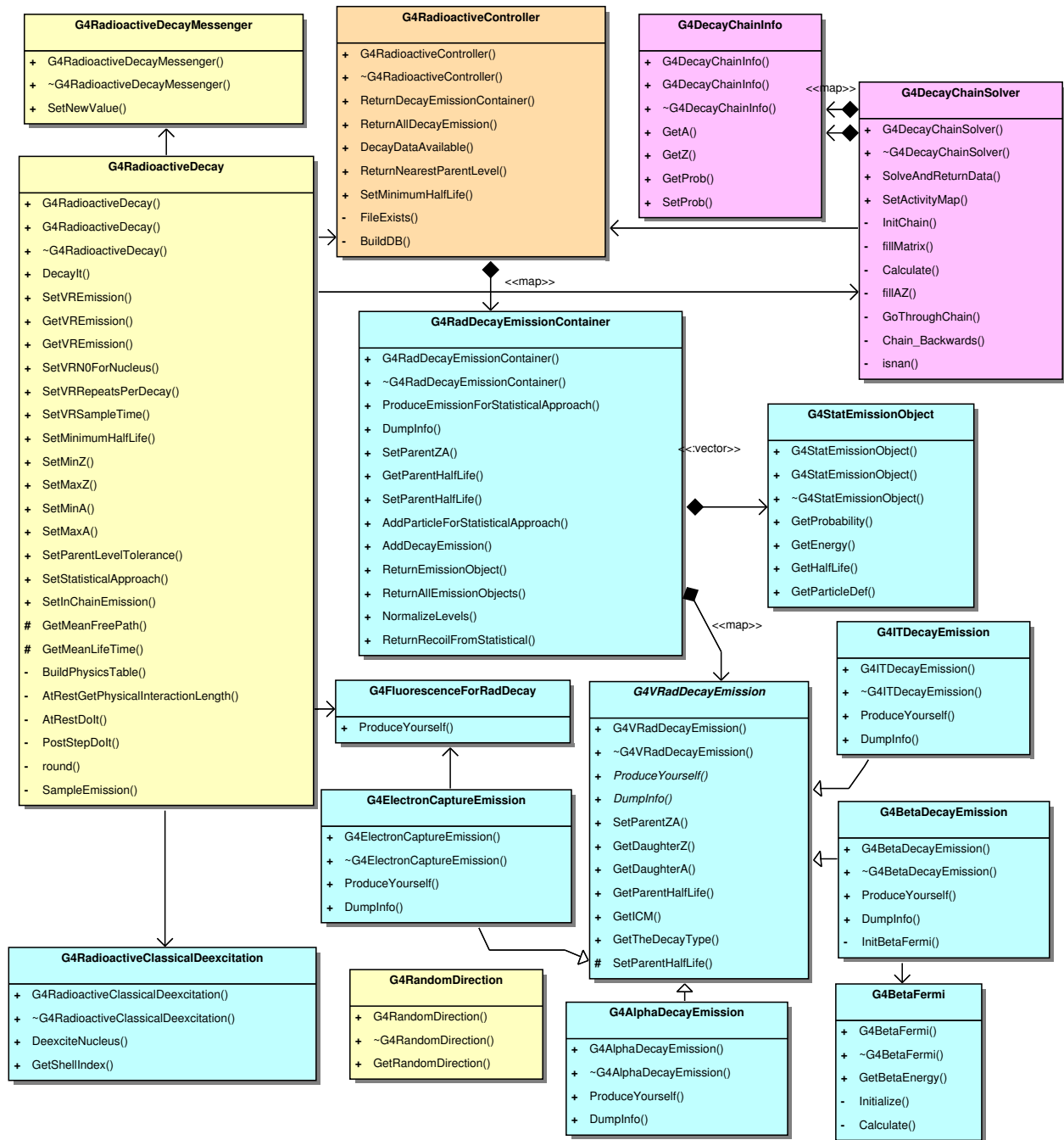
Figure 33: An UML class diagram for the new radioactive decay code showing the relations between the individual classes. The colors hint at the responsibilities and are matched to the activity diagram in Figure 34, they are: physics simulation (blue), data management and preparation (orange) and decay chain processing (purple). Each decay type is responsible for simulation its characteristic physics. The deexcitation and fluorescence emission for the statistical simulation approach (green) is produced by the G4VDecayEmission base class.
