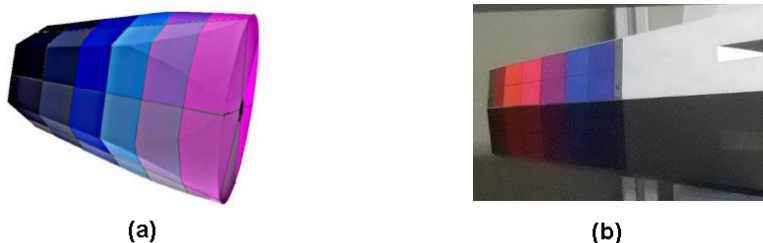
Figure 6.2.: (a) The schematic diagram of symmetric prototype AGATA crystal [17] and (b) Picture of S001 encapsulated symmetric crystal.
