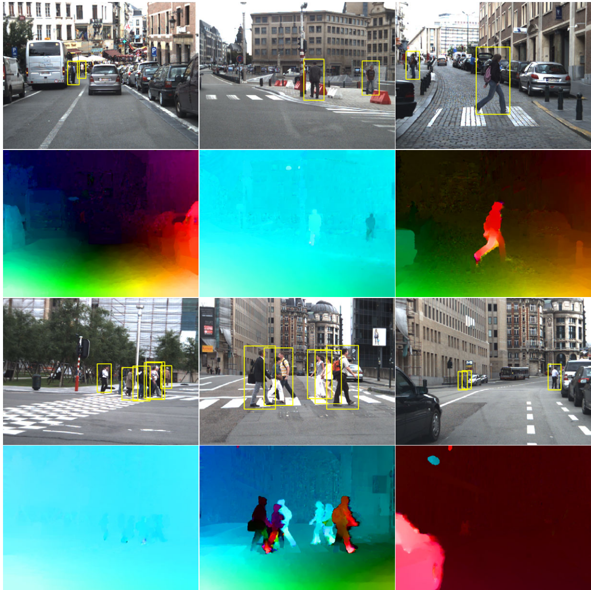
Figure 4.1: Row 1 and 3 show detections obtained with our detector in an urban environment. Row 2 and 4 show the according flow fields (Zach et al. , 2007); note the detector’s robustness to camera motion even when ego-motion dominates the optic flow field. For the optic flow color coding see Figure 4.3(b).
