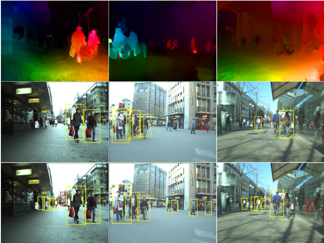
Figure 4.6: Sample detections at 0.5 FPPI on ETH-Person dataset (top row: Optic flow field of Zach et al. (2007), middle row: System of Ess et al. (2007), bottom row: Our motion-enhanced detector). Columns 1-3 correspond to Figures 4.8(e), (f) and 4.9(e) respectively, however all detections (even those smaller than 70 pixels) are shown. Note the false positive in the lower right image is actually a reflection of a true pedestrian.
