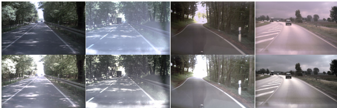
Figure 6.2: We employ a gray world assumption to normalize input images. The first image row shows unnormalized images, while the second shows the normalized results. Note that normalization yields more homogeneous images with respect to color and illumination and thus facilitates the use of texture features under challenging real-world conditions.
