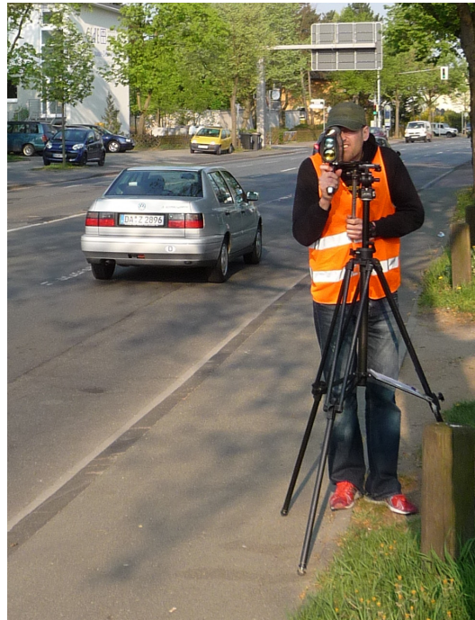
Figure 21: Speed measurement with TraffiPatrol XR
