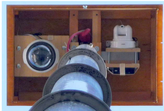
Figure 18: IP Cameras used for video observations (mounted on extension mast)
