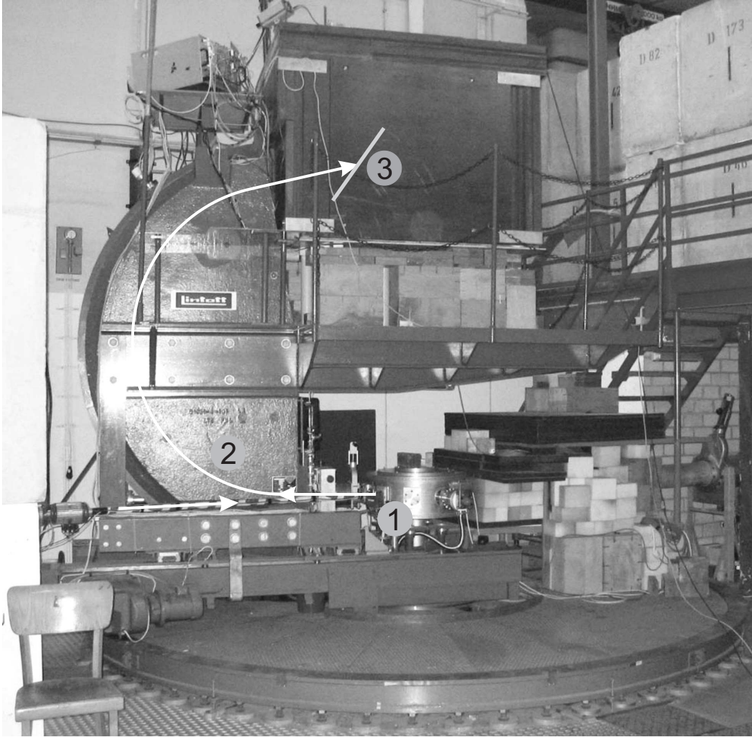
Fig. 2.3: A photo of the 169^\circ spectrometer. The electron beam goes from left to the right, hits the target placed in the scattering chamber ①. Electrons scattered in the solid angle \Omega are momentum analysed by the dipole magnet ② and focused on the focal plane ③ where the detector system is placed.
