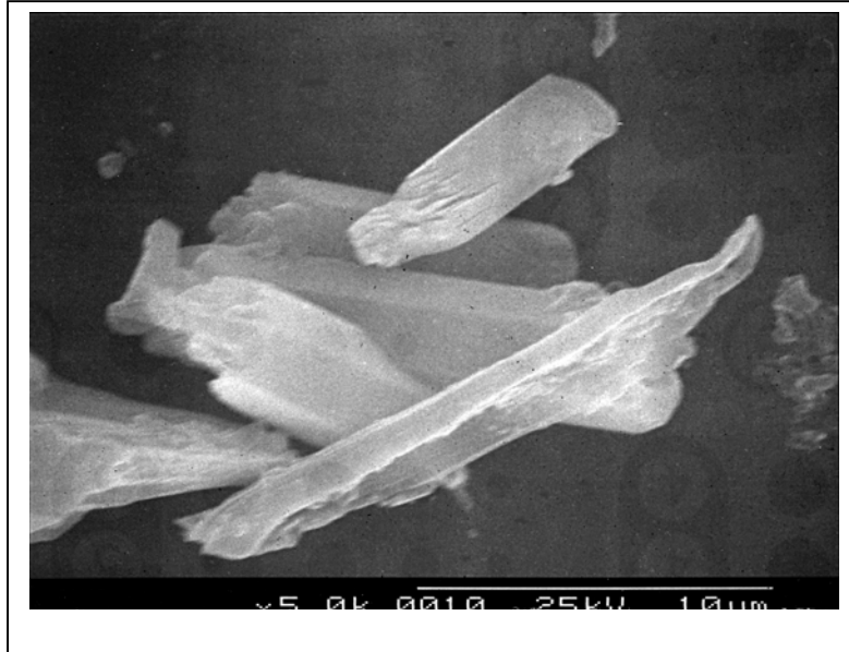
Plate 6.2 SEM photomicrograph showing the needle-like aragonite crystals of a carbonate lamina in the early-Holocene sediments.
