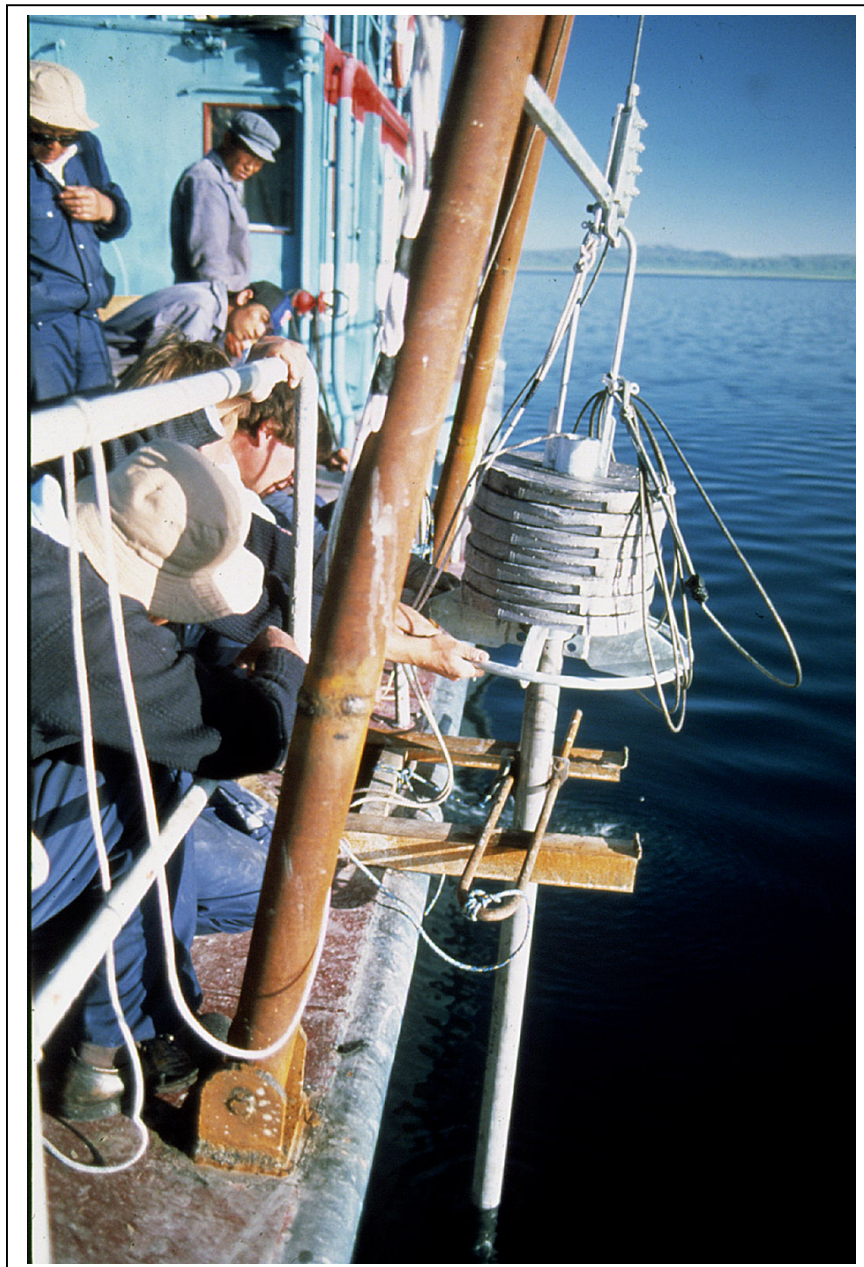
Plate 3.1 ETH Kullenberg-type corer and coring tower mounted on one side of a 30-ton ship, used for retrieving the sub-bottom sediment cores of Lake Qinghai.
