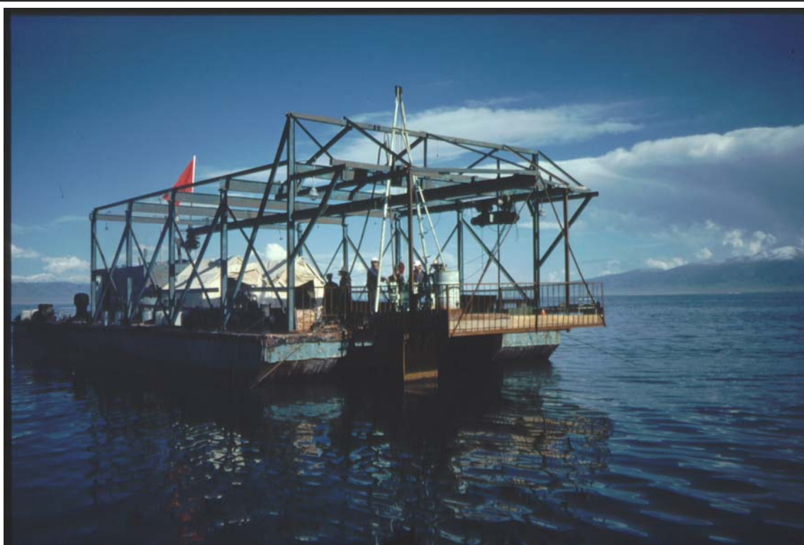
Plate 7.1 A rotary drilling rig set on a 90-ton barge fixed with 4 anchors, used for retrieving core Q87 from the water depth of 25 m in the middle of the eastern basin of Lake Qinghai.
