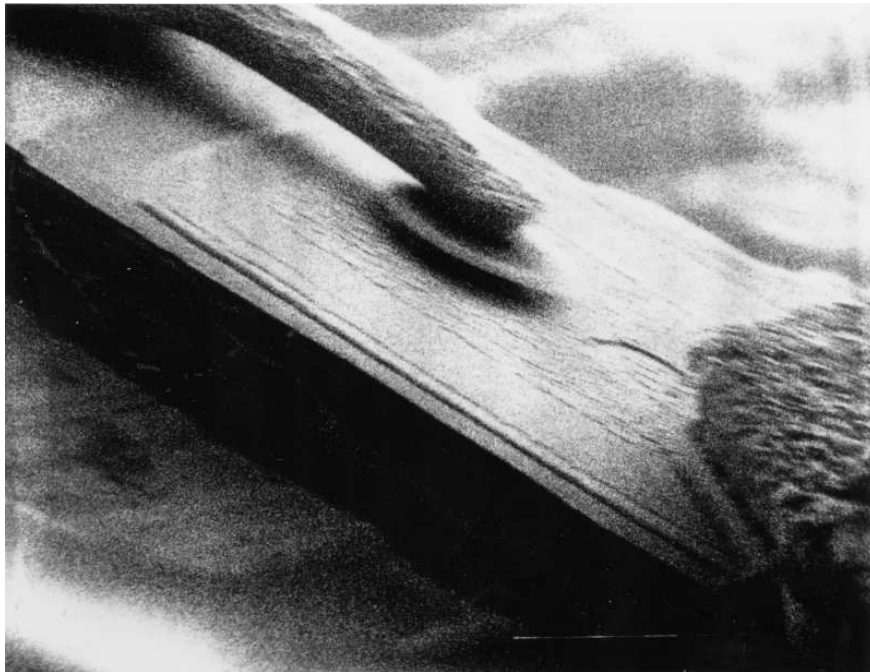
Figure 1.1: Example of a planar IHF Schottky diode.
