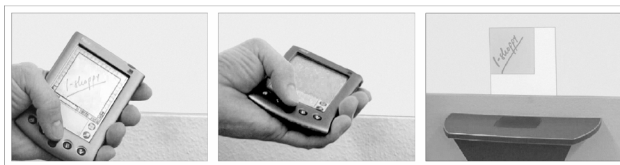
Figure 9-5. A PDA running PalmBeach pointing at an electronic whiteboard to transfer a card
