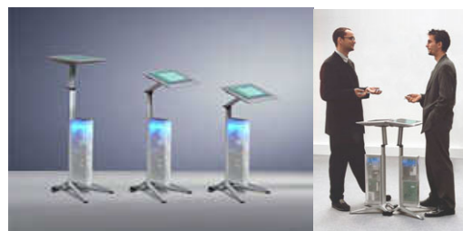
Figure 8-8. (a) Three working-modes of the ConnecTable: connect, stand-up, sitting. (b) Two connected ConnecTables.
