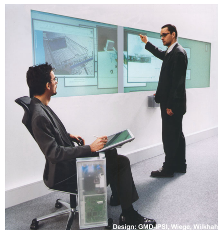
Figure 2-4. Tight collaboration, using a CommChair in front of a DynaWall. The user in the chair can remotely interact with information displayed at the wall by using the display attached to the chair. In addition, he can access his personal workspace.
