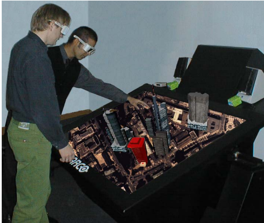
Fig. 6-4: Usage of Active Pieces for interaction at the Virtual Table (Montage: the skyscrapers in the images are manipulated to show the stereoscopic impression)
