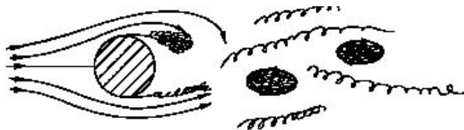
c) Turbulent flow with an agitated boundary layer: 5000 < Re < 2 \times 10^5
