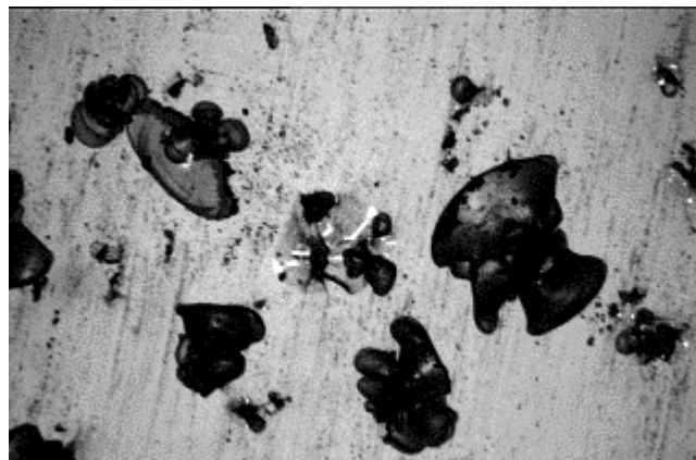
Fig. 5.1 Cracks developed on glass surface. Display extension \times 100 Source: [5.1]
