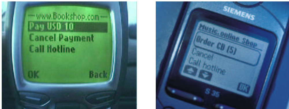
Figure 6.5: Examples of WebSIM user interaction. The pictures show how the SelectItem command is used to perform user interaction in an m-commerce setting.
