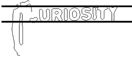
Figure 4. The edge structure on the left extends far above and below the overlapped VTB and is therefore ignored. The small edge structure on the left of the letter “U” is too small compared to the VTB height and is therefore ignored as well. All other characters are left intact.
