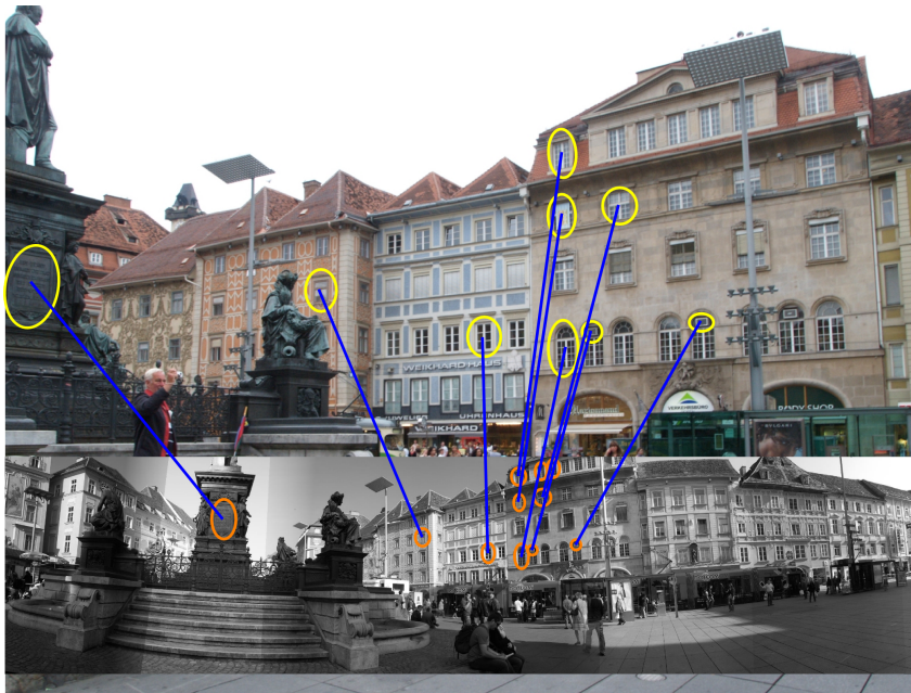
Figure 3.3: The third step of our method: Estimation of geometric relations [22]. The query image is in color, while the reference panorama is greyscale.
