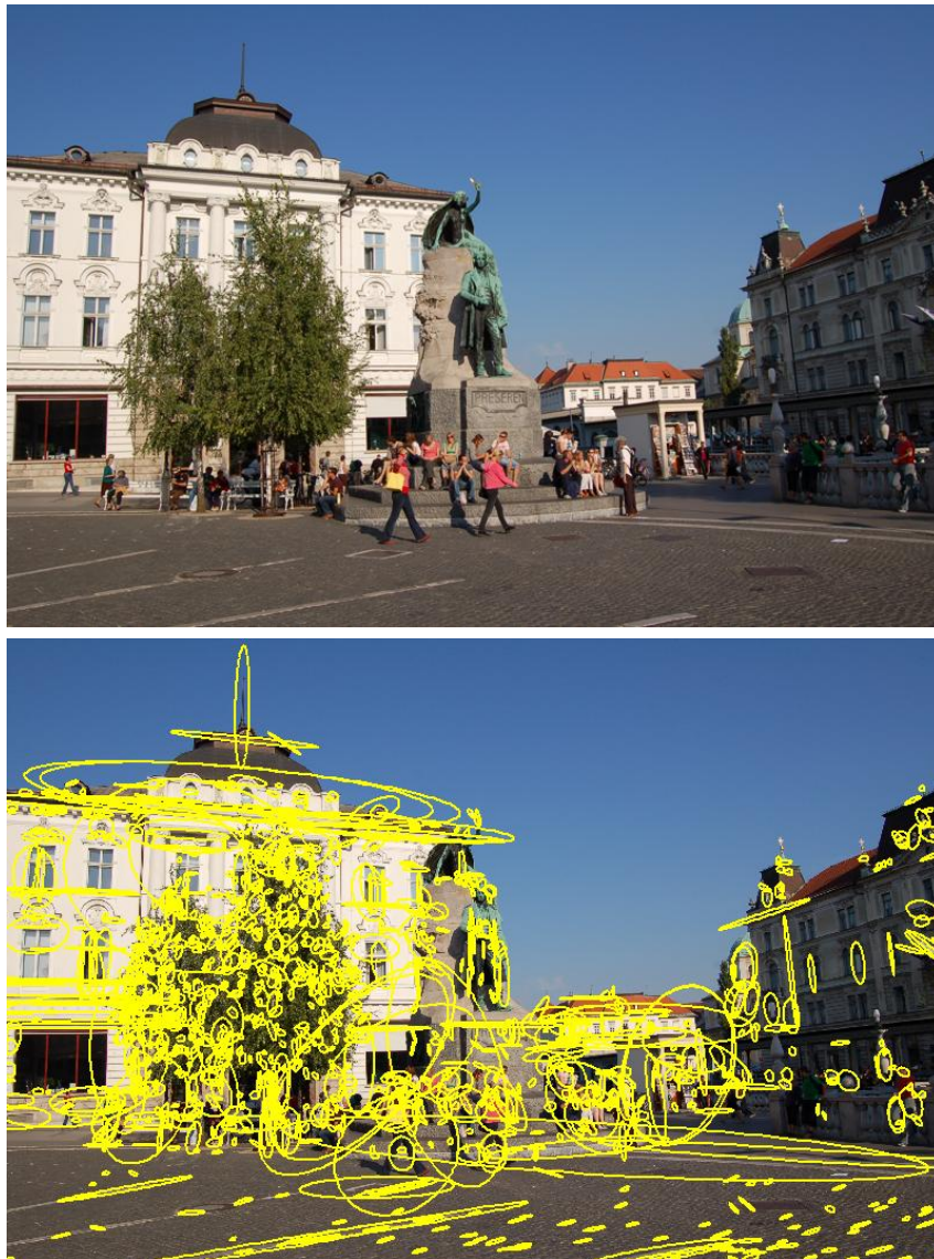
Figure 3.5: An example of detected MSER features. Top: input image. Bottom: detected MSER features. For the sake of clarity, only every fourth MSER feature is shown.
