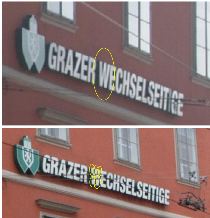
Figure 3.6: In the top image letter W is represented by a single MSER feature. In the bottom image the letter W is cut in several pieces by electric wires. While these wires have negligible effect on human recognition of the letter W, they have profound effect on automatic image matching. Due to the wires, the letter W is no longer a single connected image region of similar light intensity but is instead represented by five MSER features with each of the five features representing only a portion of the letter. Image matching based on local invariant features requires one-to-one matching between features and it cannot comprehend that the letter W in the bottom image is actually represented by five MSER features.
