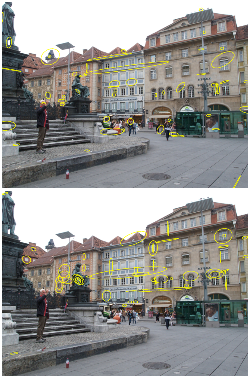
Figure 3.10: The top image depicts a random selection of 50 query features (yellow ellipses) out of 1829 features detected in this query image. The bottom image depicts 50 query features that have meaningful nearest neighbors with the highest weight among the features detected in one of the reference panoramas. Note, that the selected query features in the bottom image are more likely to represent stable visual structures such as windows, ornaments and letters, and are therefore more suitable for the image matching.
