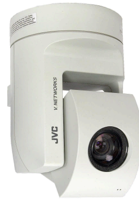
Figure 3. The JVC network camera VN-C3WU with a build-in web server is used in the latest version of the IVS system.
