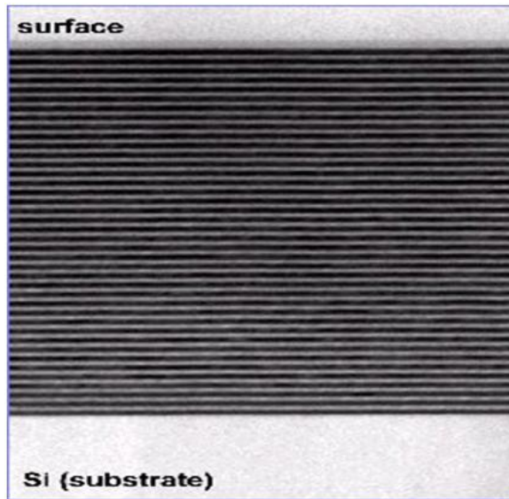
Figure 13: An image of a multilayer coating obtained by Transmission Electron Microscopy (TEM)
