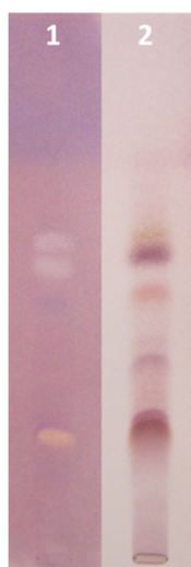
Fig. 2. TLC of DCM extract. 1: bioautography with 1-naphtyl acetate reagent, 2: derivatization with anisaldehyde-sulfuric acid. Mobile phase \text{CHCl}_3 -EtOAc-MeOH (90+7+3).
