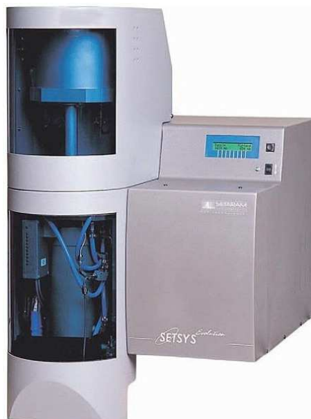
Figure 21: differential thermal analyzer Setaram SETSYS Evolution TGA & DTA 2400 [37]
