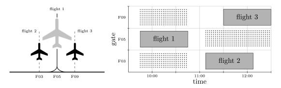
Figure 2: Example for gate shadow restrictions
