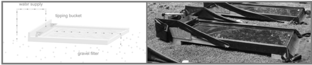
Figure 1 Schematic and photographic illustration of the algal turf scrubber construction.
