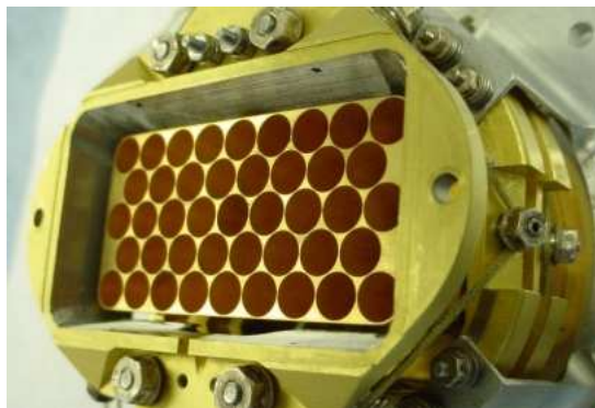
Figure 2.9: SPIRE detector 500 \mu\text{m} , 43 holes, [ESA, 2012a].
