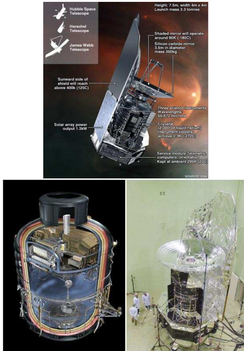
Figure 2.2: Herschel Space Telescope, artists impression, bottom left: cryo tank with focal plane units inside, bottom right: impressions from the building phase, [Pilbratt et al., 2010], [ESA, 2012a].
