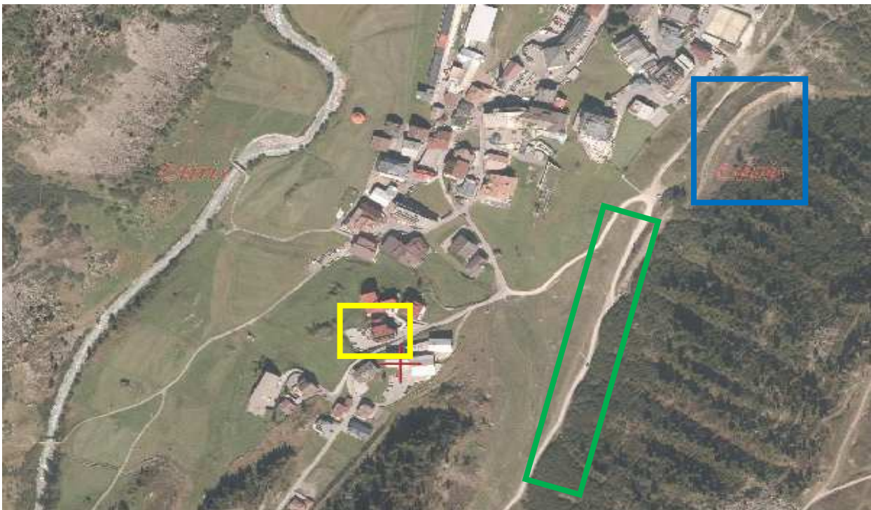
Fig. 4.4: tirisMaps image of the village Obergurgl (© 2011, tiris, BEV). The gravity measurement point is marked by the red cross. The building and parking area (yellow rectangle), the forest road (green) and the avalanche gallery (blue) are highlighted.
