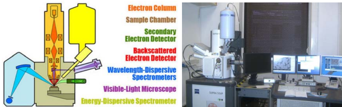
Fig. 9. Schematic cut-away diagram of a microprobe. Image courtesy of the University of Minnesota Electron Microprobe Lab (left side of the figure) [7] and overview of actual EPMA used in present research work.
