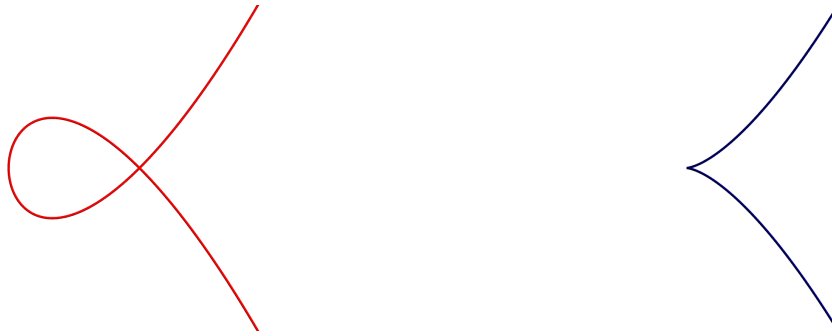
Figure B.2: the node with equation x^2 = y^2 + x^3 and the cusp x^3 = y^2 .
