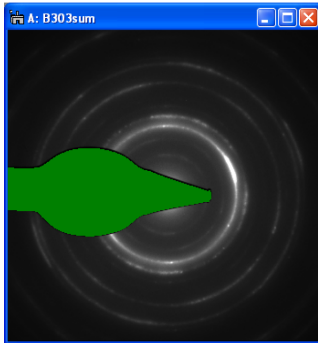
Figure 3.8: The software PASAD-tools allows to crop the beamstop.
