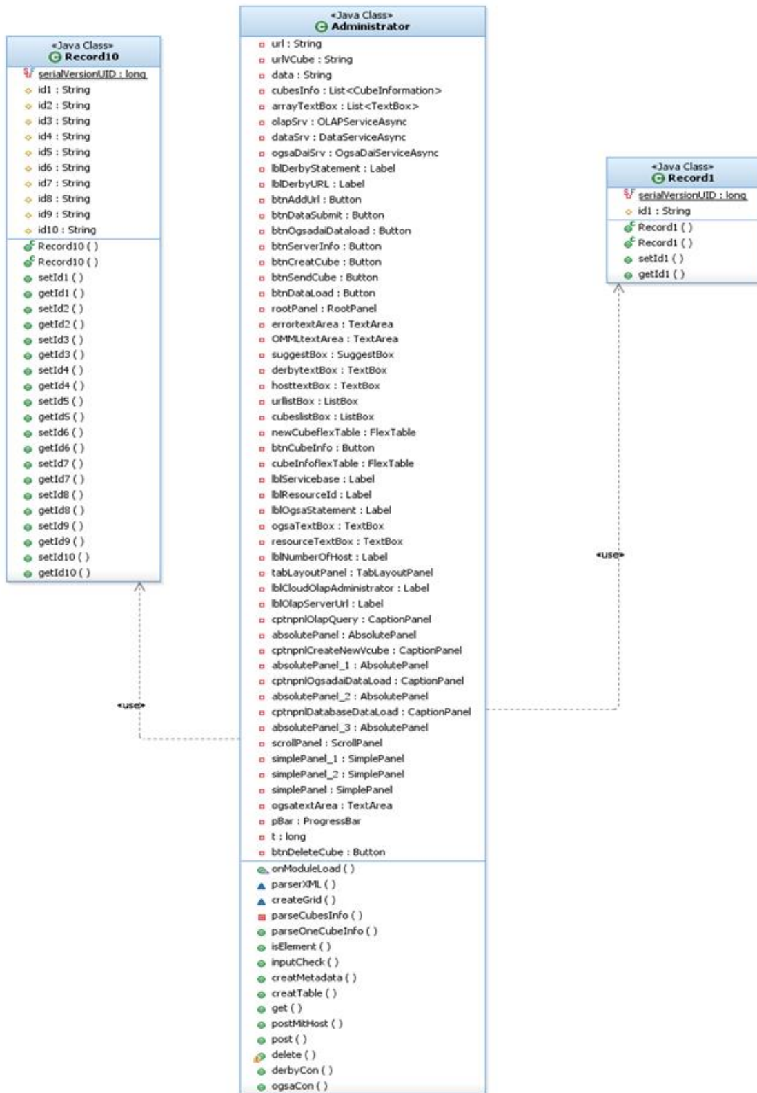
Figure C.1: Class diagram of Administrator, Record1 and Record10
