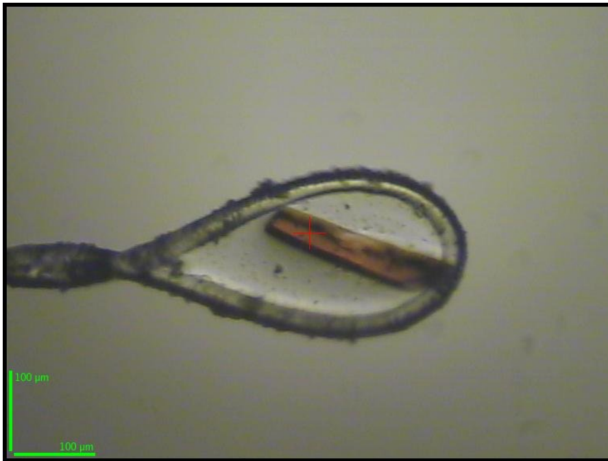
Figure 13: Crystal of NdCld mutant R173E in a nylon loop mounted on ESRF beamline BM14U. The scalebars indicate a size of 0.1 mm.
