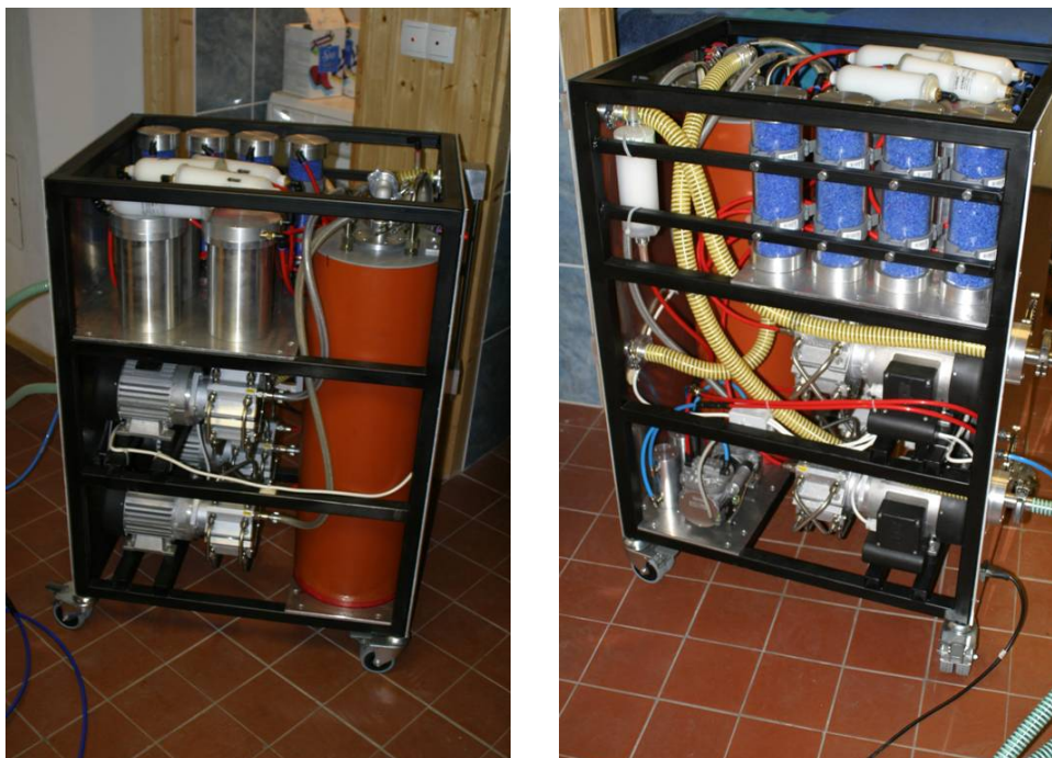
Fig. 3.3 Pictures of the first flow control unit allowing for flow rates up to 300 L/min
