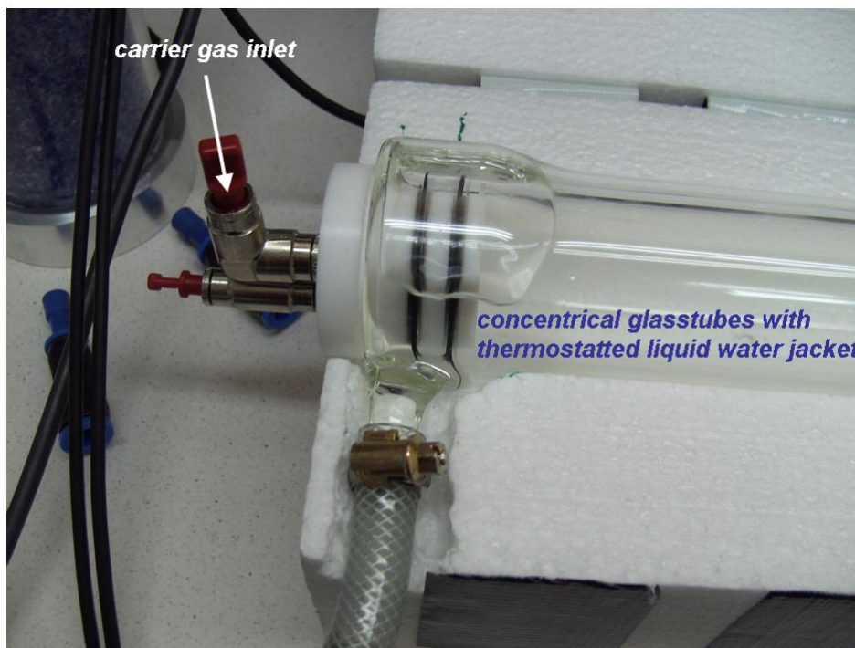
Fig. 4.36 Close up of the custom-built humidifier
