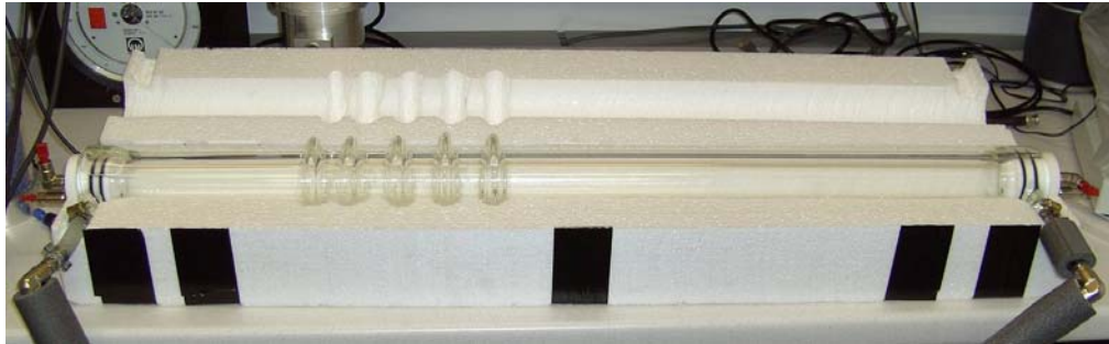
Fig. 4.37 Humidifier in its polystyrene housing
