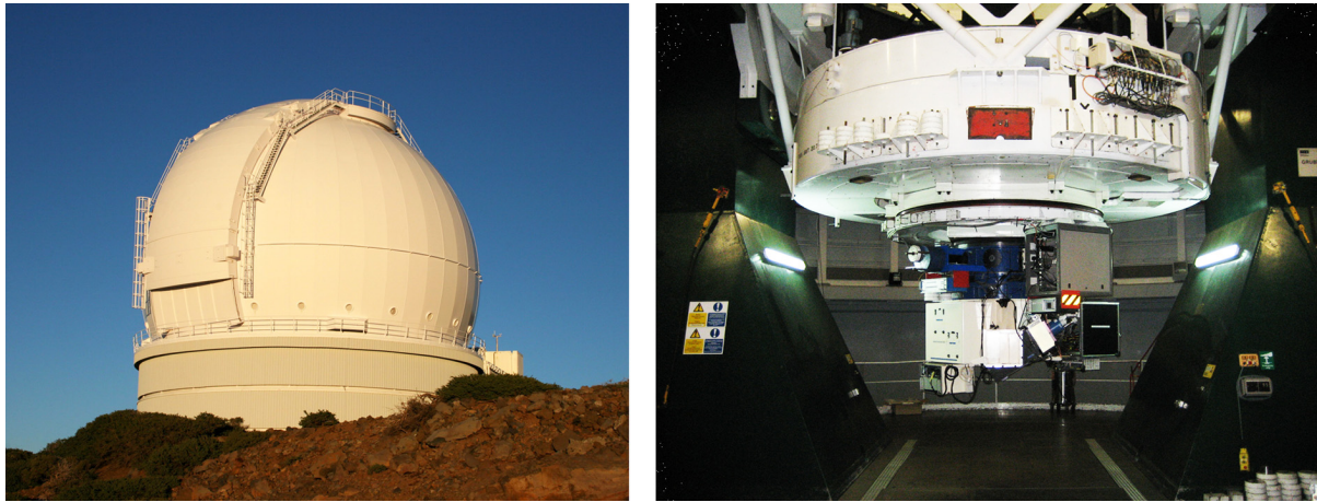
Figure 3.1: Left panel: The William Herschel Telescope (WHT) located on the Roque de los Muchachos on the edge of the Caldera de Taburiente National Park, 2396 meters above sea level. Photo Courtesy of the Isaac Newton Group of Telescopes, La Palma. Right panel: ISIS mounted at the cassegrain focus of the WHT. Private photograph.
