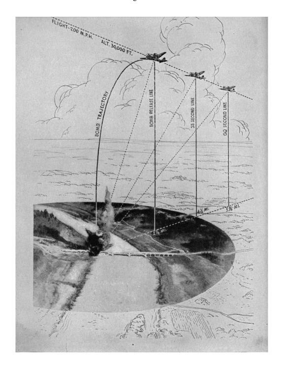
'Precision bombing diagram. Bombardier must see the target and have bomb sight in operation at 35-second line for precision bombing. Greater accuracy is possible if target can be seen from the 60-second line.' (Robert Breckenridge, 1942)
