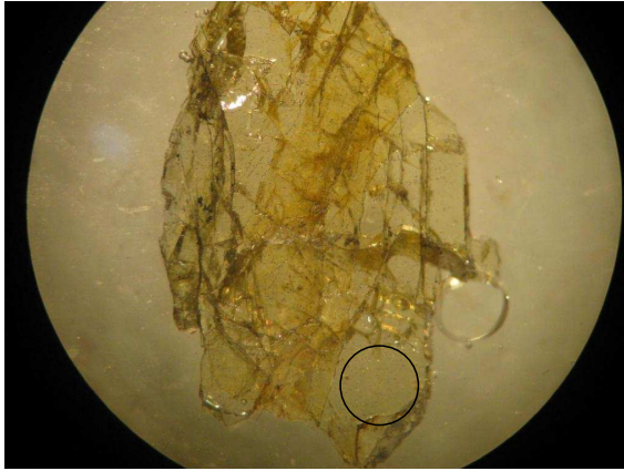
Fig. 8. Platelet of the Fe-rich Sri Lanka sample used for transmission measurements under polarized light. The sample has a width of 4 mm and a length of 6 mm. The black circle features the spot of the measurements.
