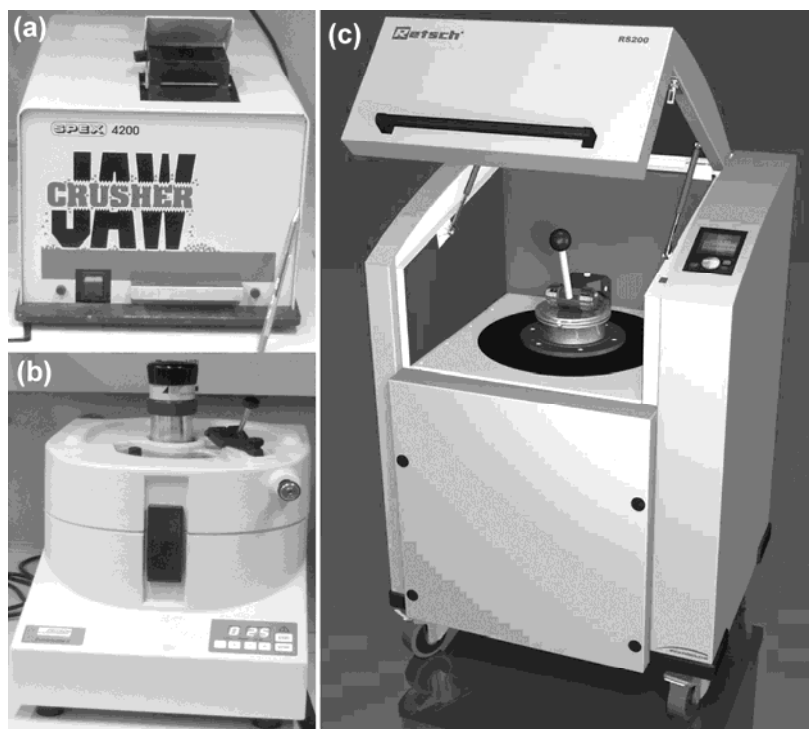
Figure 3.1 Powdering machines of the Department of Lithospheric Research: (a) Jaw crusher; (b) Mechanical agate mill, and (c) Vibratory disk mill.
